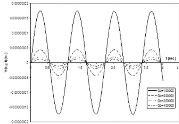
**Fig. 5.4.** Displacement profile of simply supported rectangular plate on variable Pasternak foundation and traversed by moving force for  $F_0 = 100000$ ,  $R_0 = 0.4$  and various values of  $G_0$ .
