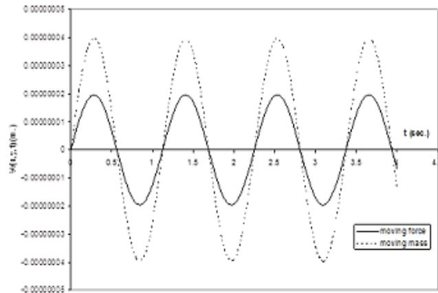
**Fig. 5.9.** Comparison of deflection of moving force and moving mass cases for simply supported rectangular plate on variable Pasternak foundation and traversed by moving force for  $F_0 = 1000000$ ,  $G_0 = 100000$  and  $R_0 = 0.4$ .
