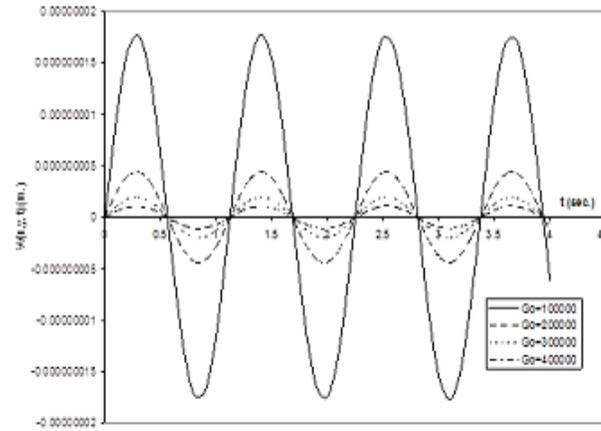
**Fig. 5.3.** Displacement profile of simply supported rectangular plate on variable Pasternak foundation and traversed by moving force for  $F_0 = 0$ ,  $R_0 = 0.4$  and various values of  $G_0$ .
