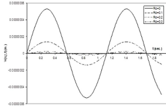
**Fig. 5.2.** Deflection profile of simply supported rectangular plate resting on variable Pasternak foundation and traversed by moving force for  $F_0 = 2000000$ ,  $G_0 = 900000$  and various values of  $R_0$
