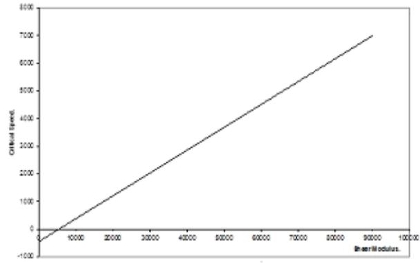
**Fig. 5.10.** Graph of Critical Speed against Shear Modulus.
