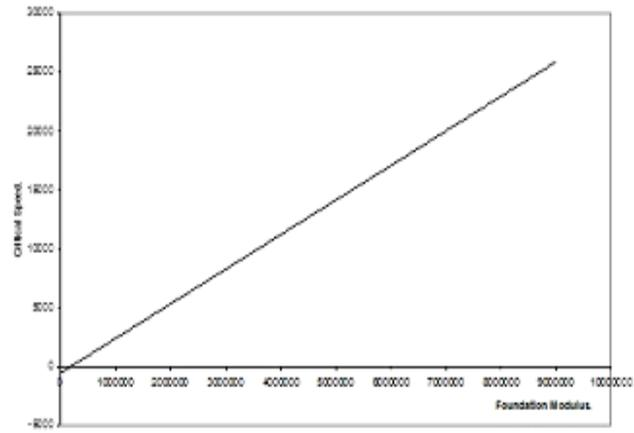
**Fig. 5.11.** Graph of Critical Speed against Foundation Modulus.
