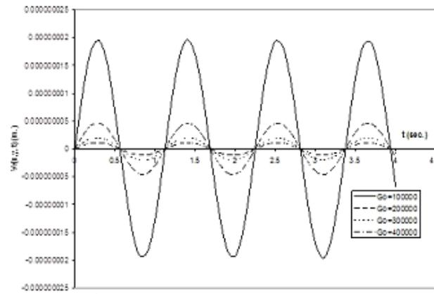
**Fig. 5.5.** Displacement profile of simply supported rectangular plate on variable Pasternak foundation and traversed by moving force for  $F_0 = 1000000$ ,  $R_0 = 0.4$  and various values of  $G_0$ .
