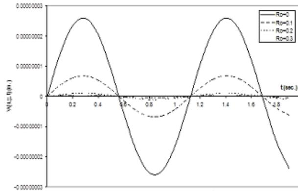
**Fig. 5.1.** Deflection profile of simply supported rectangular plate on variable Pasternak foundation and traversed by moving force for  $F_0 = 2000000$ ,  $G_0 = 900000$  and various values of  $R_0$
