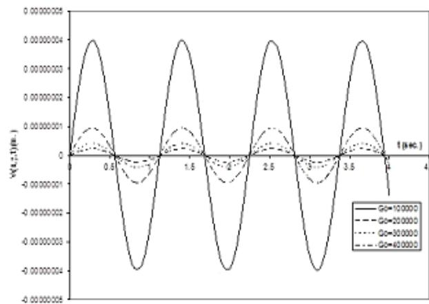
**Fig. 5.6.** Displacement profile of simply supported rectangular plate on variable Pasternak foundation and traversed by moving mass for  $F_0 = 0$ ,  $R_0 = 0.4$  and various values of  $G_0$ .
