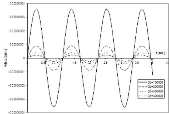
**Fig. 5.7.** Deflection of simply supported rectangular plate resting on variable Pasternak foundation and traversed by moving mass for  $F_0 = 100000$ ,  $R_0 = 0.4$  and various values of  $G_0$ .
