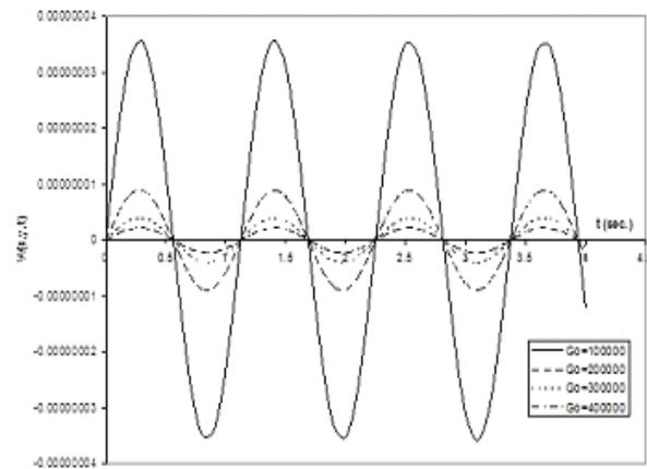
**Fig. 5.8.** Deflection of simply supported rectangular plate on variable Pasternak foundation and traversed by moving mass for  $F_0 = 1000000$ ,  $R_0 = 0.4$  and various values of  $G_0$ .
