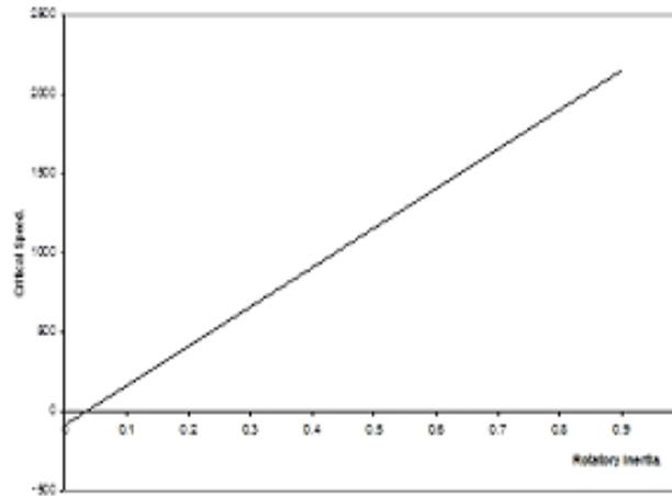
**Fig. 5.12.** Graph of Critical Speed against Rotatory Inertia.
