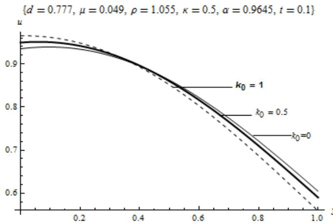
**Figure 1.** Effect of taper parameter on velocity profile
