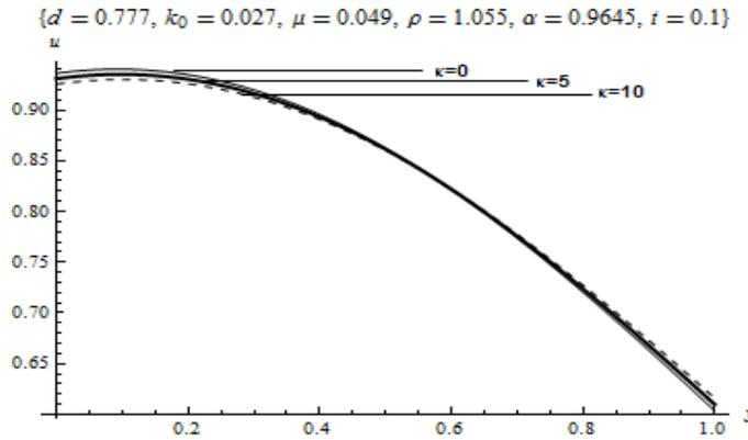
Figure 3. Effect of elasticity parameter on velocity profile
