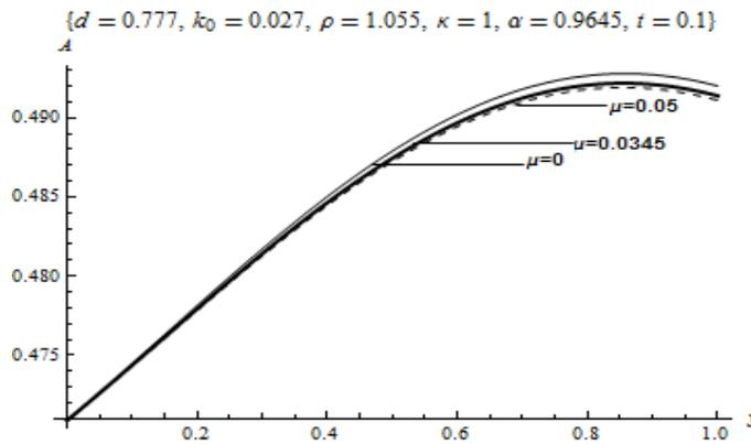
Figure 4. Effect of dynamic viscosity on arterial cross sectional area
