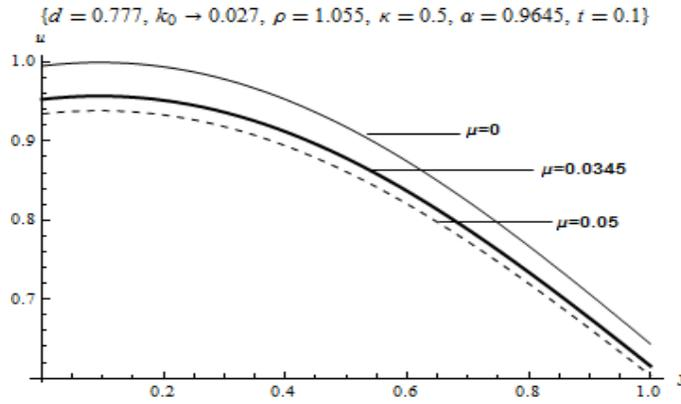
Figure 2. Effect of dynamic viscosity on velocity profile
