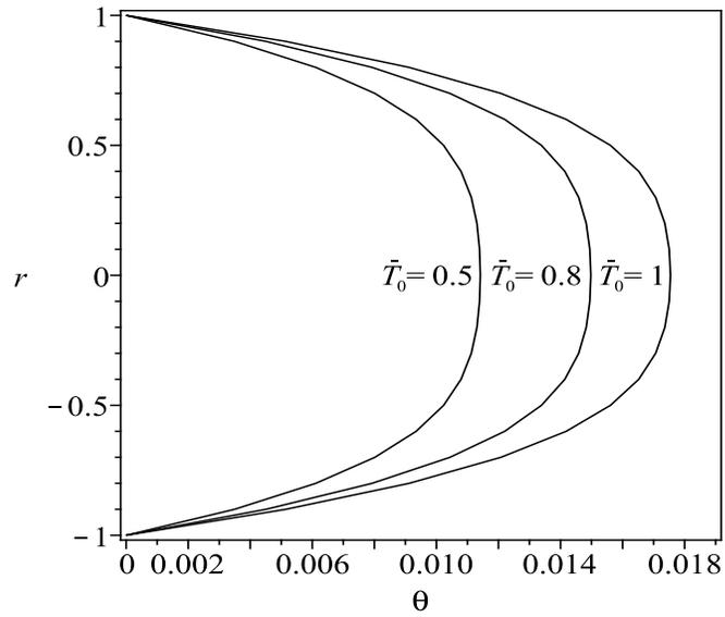
**Fig. 10.** Effect of initial temperature  $\bar{T}_0$  on the picture of radius  $r$  on the temperature distribution  $\theta$  of Vogel's viscosity model with  $A = B = -C = \Gamma = \Lambda = \delta = 1$ .
