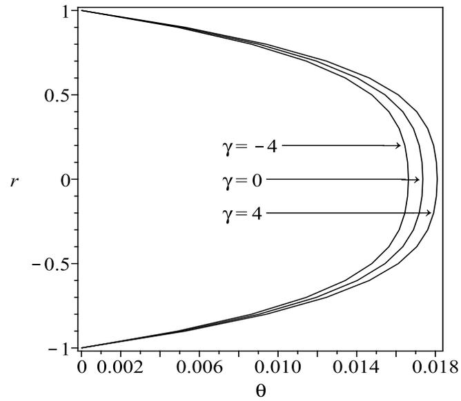
**Fig. 6.** Temperature distribution of Reynold's viscosity model for different values of  $\gamma$  with  $\Gamma = \Lambda = \delta = -C = 1$ .
