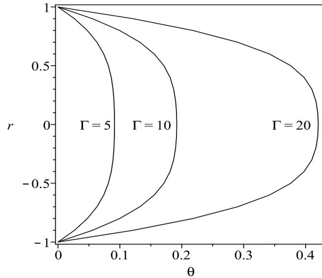
**Fig. 12.** Effect of viscous dissipation parameter  $\Gamma$  on the dependence of radius  $r$  on the temperature distribution  $\theta$  of Vogel's viscosity model with  $A = B = -C = \bar{T}_0 = \Lambda = \delta = 1$ .
