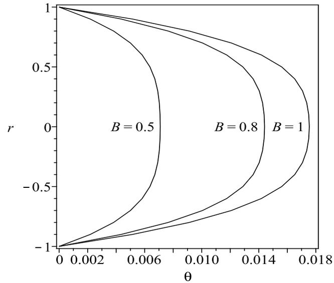
**Fig. 8.** Effect of the parameter  $B$  on variation of radius  $r$  with the temperature  $\theta$  of Vogel's viscosity model with  $A = -C = \bar{T}_0 = \Gamma = \Lambda = \delta = 1$ .
