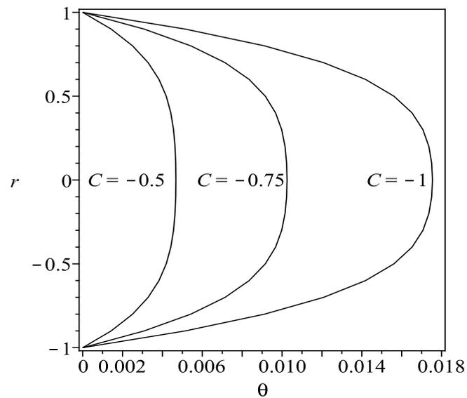
**Fig. 9.** Effect of the dimensionless pressure gradient  $C$  on the curve of radius  $r$  with the temperature  $\theta$  of Vogel's viscosity model with  $A = B = \bar{T}_0 = \Gamma = \Lambda = \delta = 1$ .
