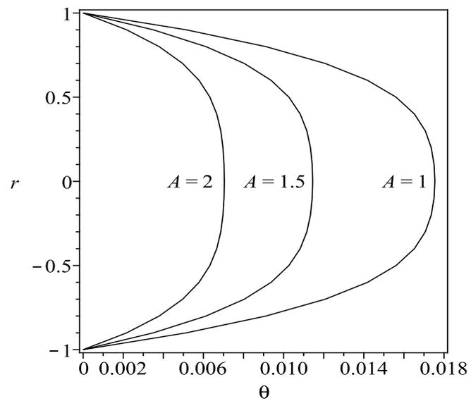
**Fig. 7.** Effect of the parameter  $A$  on graph of radius  $r$  with the temperature  $\theta$  of Vogel's viscosity model with  $B = -C = \bar{T}_0 = \Gamma = \Lambda = \delta = 1$ .
