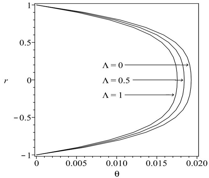
**Fig. 11.** Effect of Non-Newtonian parameter  $\Lambda$  on the plot of radius  $r$  versus the temperature distribution  $\theta$  of Vogel's viscosity model with  $A = B = -C = \bar{T}_0 = \Gamma = \delta = 1$ .
