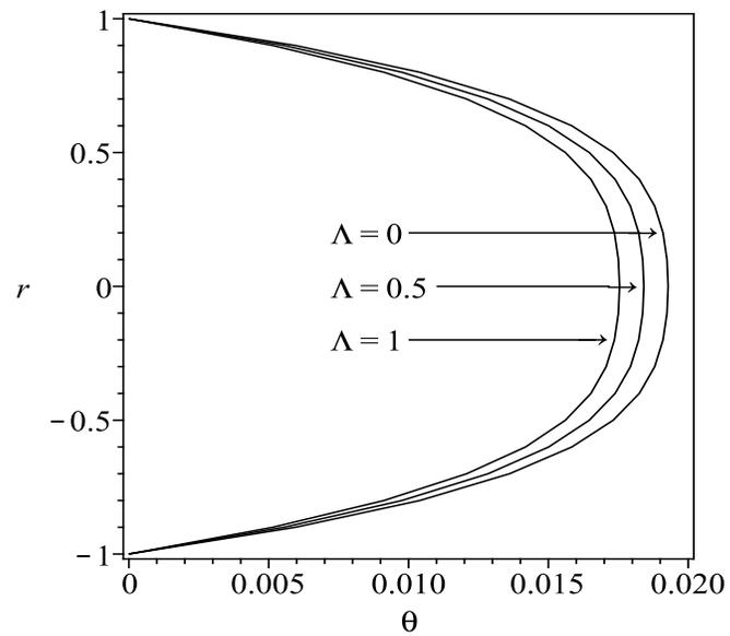
**Fig. 3.** Radius  $r$  versus temperature  $\theta$  of Reynold's viscosity model for values of  $\Lambda$  when  $\Gamma = \gamma = \delta = -C = 1$ .
