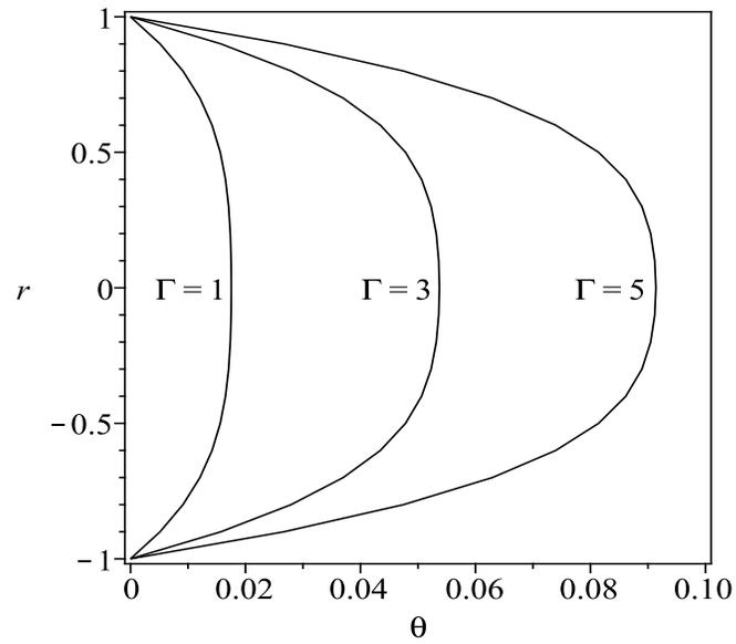
**Fig. 4.** Radius  $r$  versus temperature  $\theta$  of Reynold's viscosity model for values of  $\Gamma$  when  $\Lambda = \gamma = \delta = -C = 1$ .
